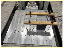
Random Vibration Test: Y axis/ Mechanical Shock Test: ±Y axis
