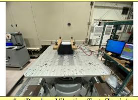
Random Vibration Test: Z axis/ Mechanical Shock Test: ±Z axis
